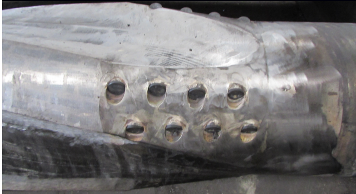
Figure 3. Close up of TCI Stud Cutters on PDC Reamer
