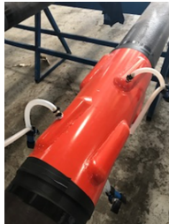
Patented Swellable Packer and End Ring Technology
